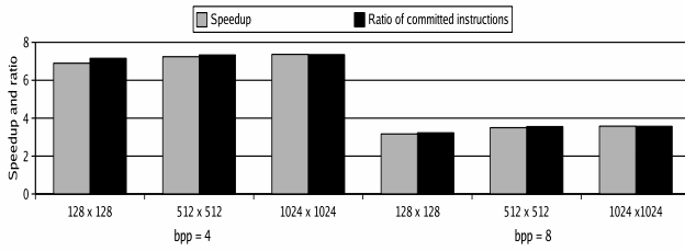
Figure 6. Speedup and ratio of committed instructions of the 8-way hierarchical structure over the fully scalar implementation for different image sizes and bpps on the single issue processor.
