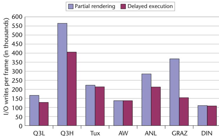
**Figure 8.** Average number of state information writes to the accelerator per frame on the GraalBench benchmark suite.
