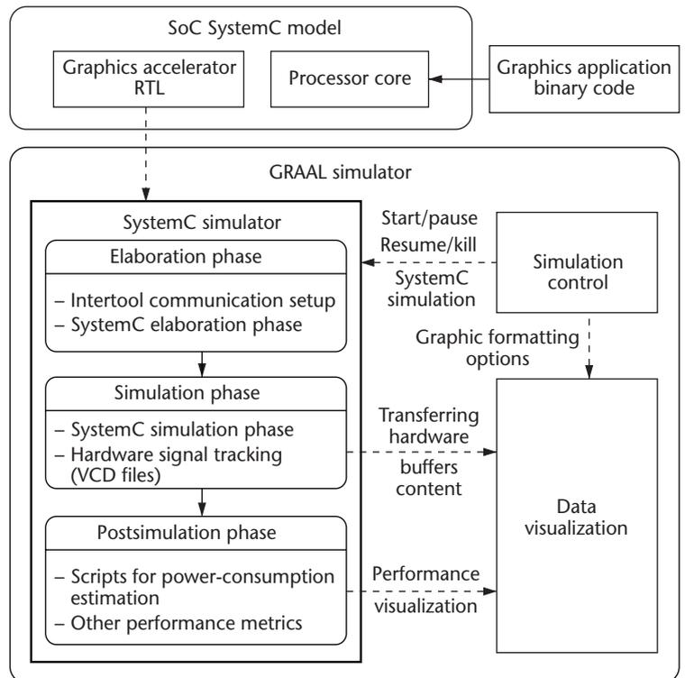
**Figure 2. The GRAAL simulator framework. The framework integrates SystemC simulation together with simultaneous graphics visualization and performance estimation.**
