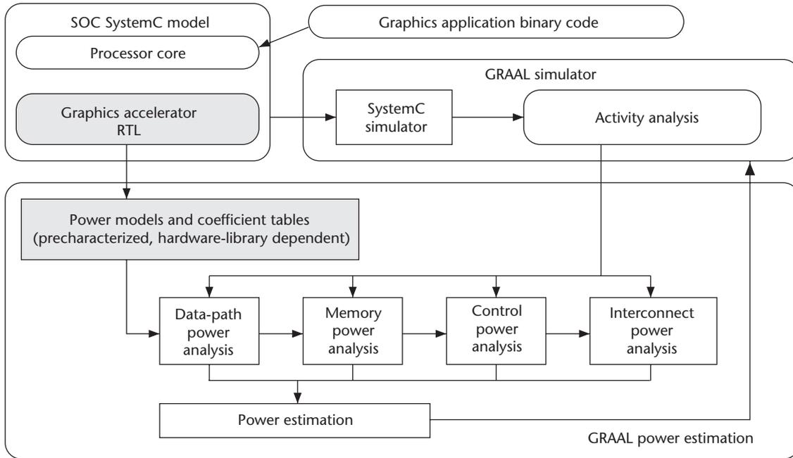
**Figure 10.** GRAAL architecture-level power estimation strategy. Template circuit classes derived from power-precharacterized hardware modules are used together with signal activities to estimate power consumption.
