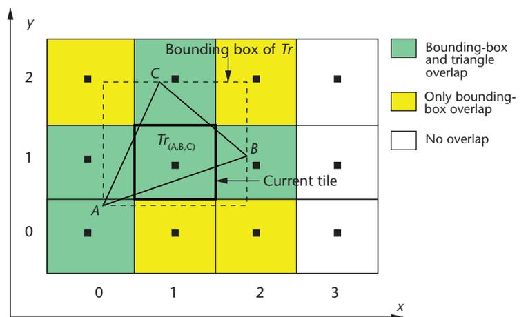
**Figure 5. Imprecision in the triangle-to-tile bounding-box (BBOX) test. In this case, the BBOX overlaps the yellow tiles but the triangle doesn't.**
