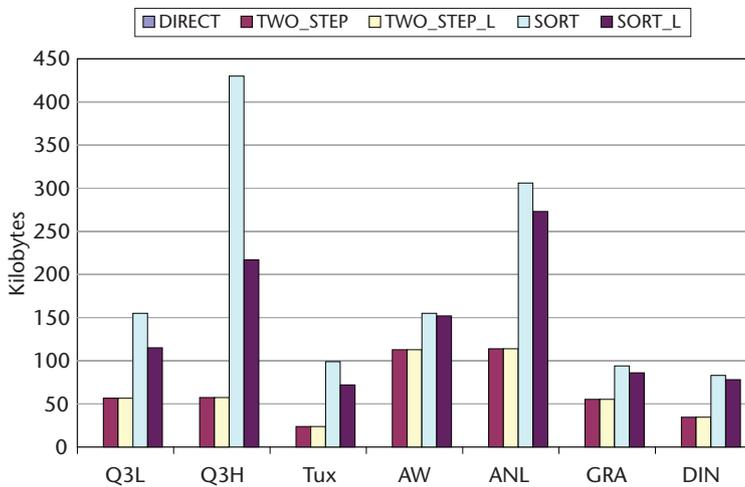
Figure 7. Memory requirements of the scene-management algorithms. The additional memory required for benchmarks with a small overlap factor (such as AW) is insignificant, but it's considerable for benchmarks with a large overlap factor (such as Q3H).
