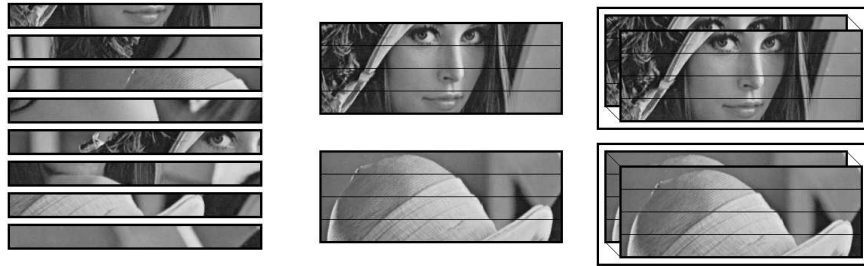
(a) Eight 1D MDSC blocks. (b) Two 2D MDSC blocks, four lines high. (c) Two 3D MDSC blocks, four lines high and 2 images deep.
